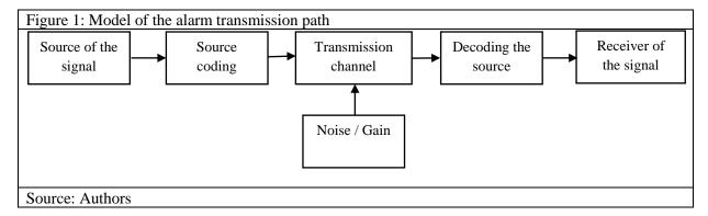
The types of transmitted signals in alarm transmission systems are divided into two groups:
